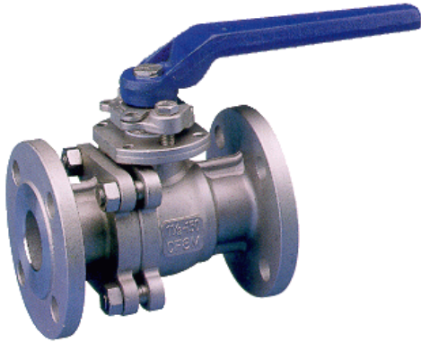
FIG. V-2F Class 150, Class 300 - 2 piece 316 Stainless steel body & trim.
