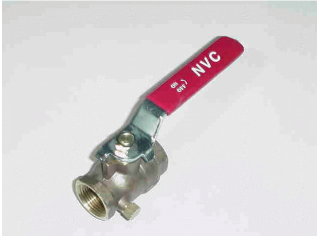
FIG: 320T- E 2 piece, Full Port Ball valve, 600# WOG, NPT ends, PTFE seats c/w Drain
