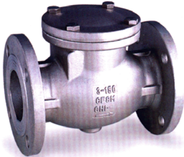
FIG. 150SC Class 150, Flanged ends, Bolted cover, 316 Stainless steel body & trim.
